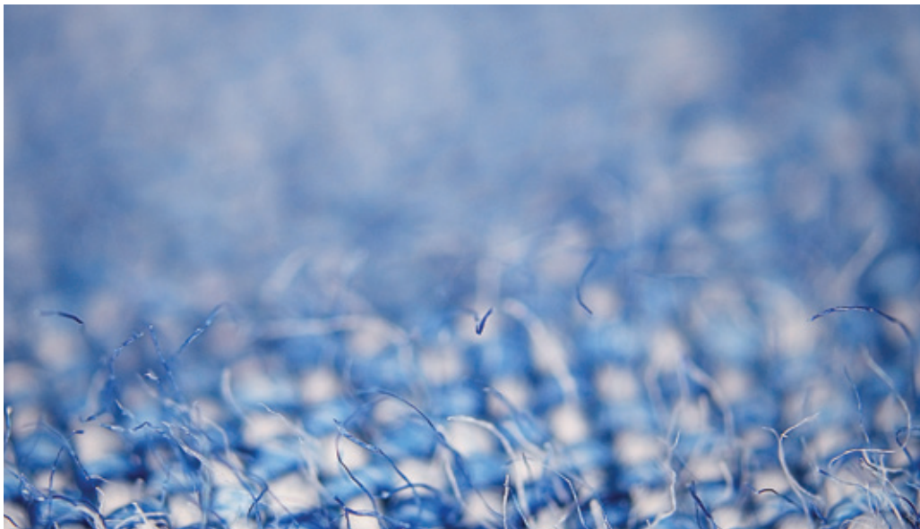
Microfibers in blue jeans. Jeans are made from both cotton and synthetic textiles. Microplastics, like these fibres, may be released from use and washing of synthetic textiles.
