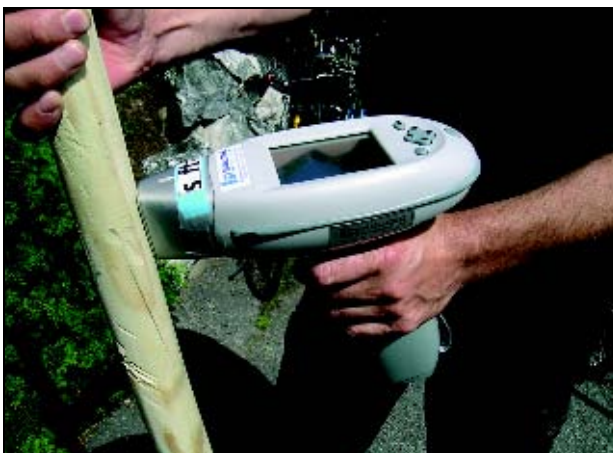
Figure 11.2 Measuring the heavy metal content of impregnated timber
