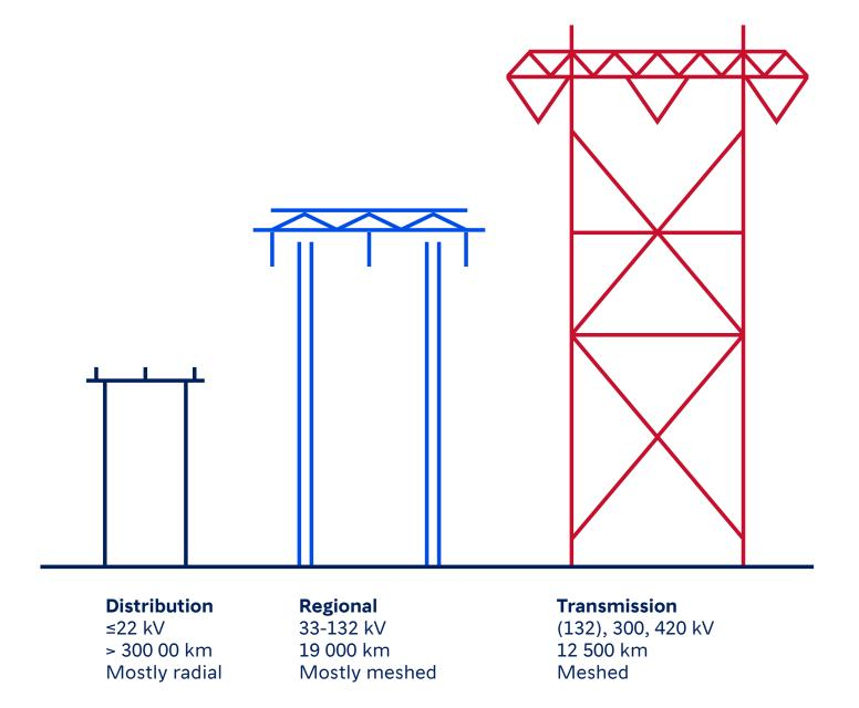
**Figure 2** The Norwegian electricity grid system. Source: NVE
