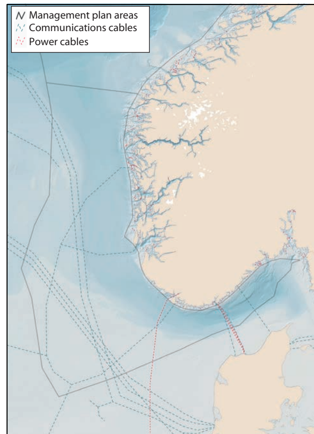
Figure 7.5 Submarine communications and power cables.
