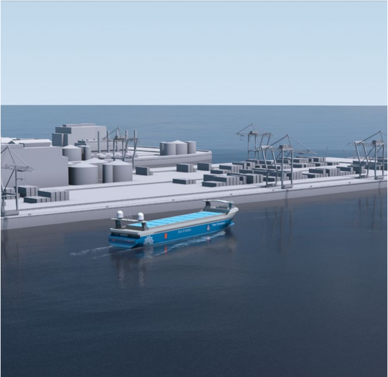
The Yara Birkeland is an autonomous electric container vessel that will be able to replace about 40 000 truck journeys per year between Yara's fertiliser plant on Herøya and Brevik and Larvik, which are the ports of shipment. Illustration: Kongsberg/Sintef
